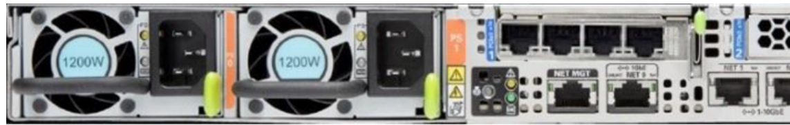
Figure 3-14 Connecting to USB and SER MGT (COM1) Ports
