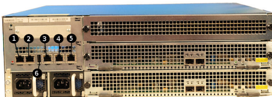
Figure A-5 Acme Packet 6300/6350 Management Interfaces
