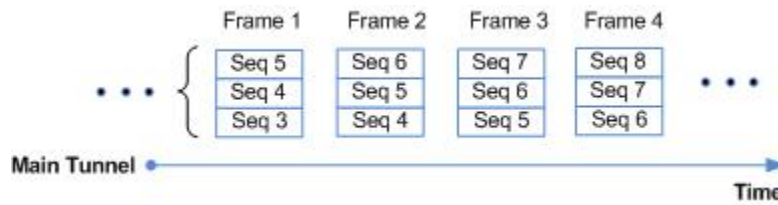
Figure 21-16 Redundancy — DTLS/UDP Redundancy
