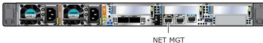
Figure 3-4 Connecting to ILOM over the Network
