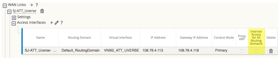
Figure 8: Enabling Internet access for All Routing Domains
