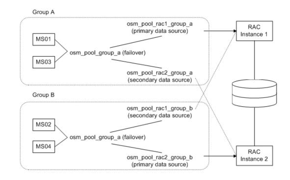
Figure 7-2 OSM Data Source Configuration for Active-Active Oracle RAC
