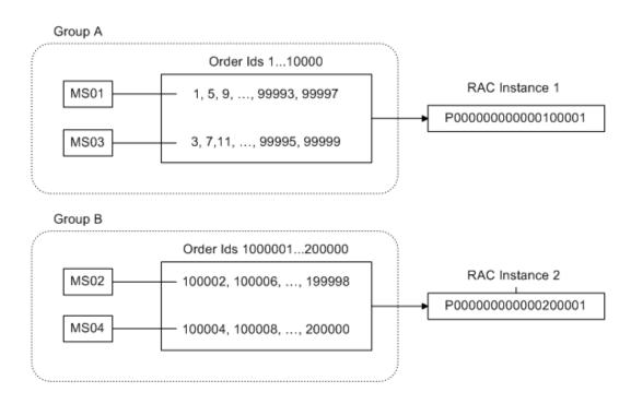
The downside of creating orders concurrently in N partitions is that some order Ids are skipped, which causes partitions to be only partially filled when they are considered exhausted. For example, Figure 3 shows that MS01 and MS03 skip order Ids 2, 6, 10, 14, and so on. This is because these are mapped to slots owned by MS02 and MS04. However, MS02 and MS04 do
