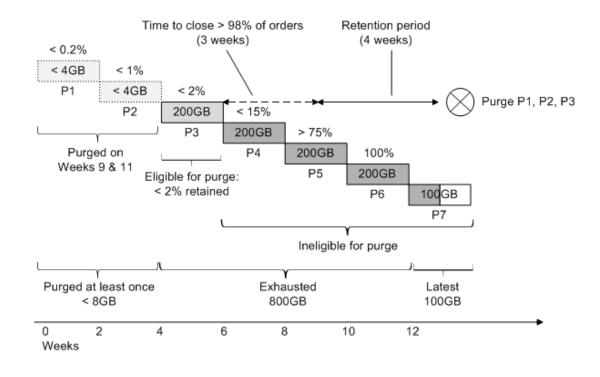
Figure 7-8 Estimating Minimum Space Consumption
