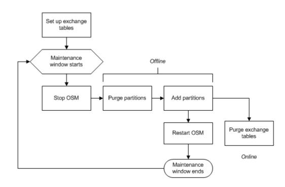
Figure 7-15 Typical Maintenance Using Partition-Based Order Purge
