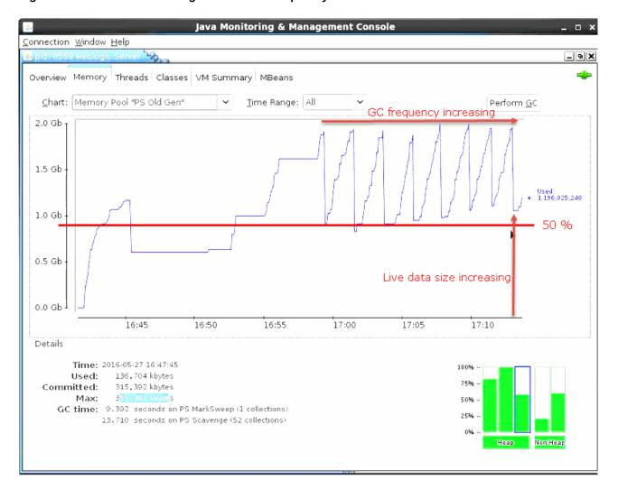
Figure 10-2 JConsole Garbage Collection Frequency and LDS Size
