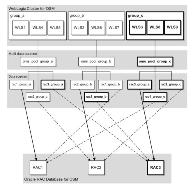
Figure 7-6 Data Sources for a Third Active Oracle RAC Instance in an Active-Active Environment
