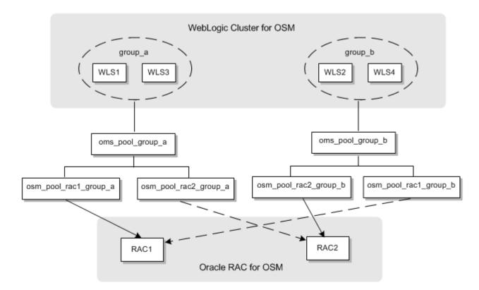
Figure 7-4 Data Source Configuration for Oracle RAC Active-Active
