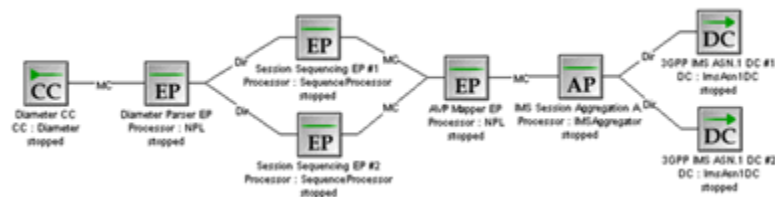
Figure 5-3 Node Chain Routing - Alternate Configuration
