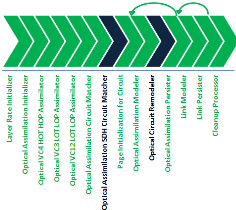
Figure 2-3 Assimilate SDH Optical Circuits Action Processor Workflow
