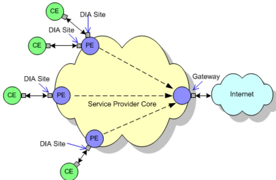
A Layer 3 interface is configured or created and placed in a DIA site. In a managed CE service, the CE device is also placed in the DIA site. IP routing is configured on the PE to route Internet traffic across the provider core to the Internet gateway and on to the Internet. Additionally, prefix lists may be configured to filter routing updates.
