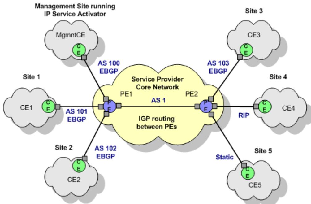
Between the management site and the core network, two links are required, one to provide VPN connectivity and one to provide routes to the Service Provider backbone IGP. These links are illustrated in [Figure 10-2](#).
