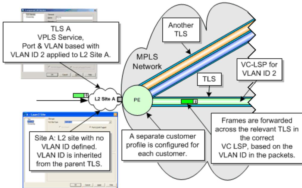
At minimum, a layer 2 site may contain a single port – represented by an Access interface on a Gateway (PE) device in the user interface. IP Service Activator configures the port as:
