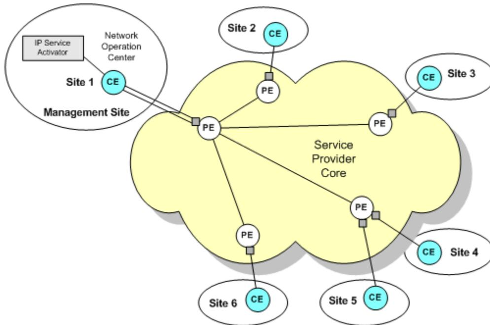
In IP Service Activator, a VPN is always associated with a customer object. One technique is to create a Customer named 'Management' and create the management VPN beneath this. Then create the 'real' Customer which maps to the real-world customer, and create a hub and spoke or fully-meshed VPN.
