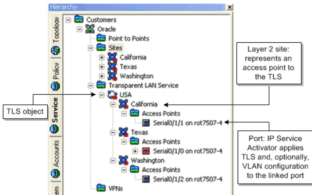
IP Service Activator represents a layer 2 port as an interface object in the client. In the descriptions that follow, the term 'interface' is used when referring to TLS setup through the client.
