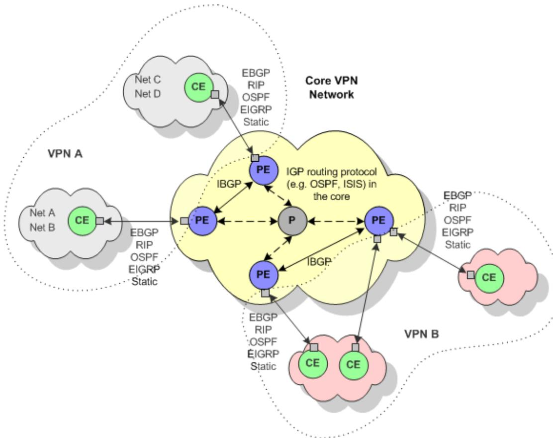
A BGP autonomous system is a collection of networks. Each autonomous system is identified by an autonomous system number (ASN), which is required when running BGP. In order to configure BGP, you need to assign an ASN to each customer site network, in addition to the service provider core network. eBGP is a variant of BGP that connects the Provider Edge (PE) router to a Customer Edge (CE) router where both the provider and customer networks are running iBGP.
