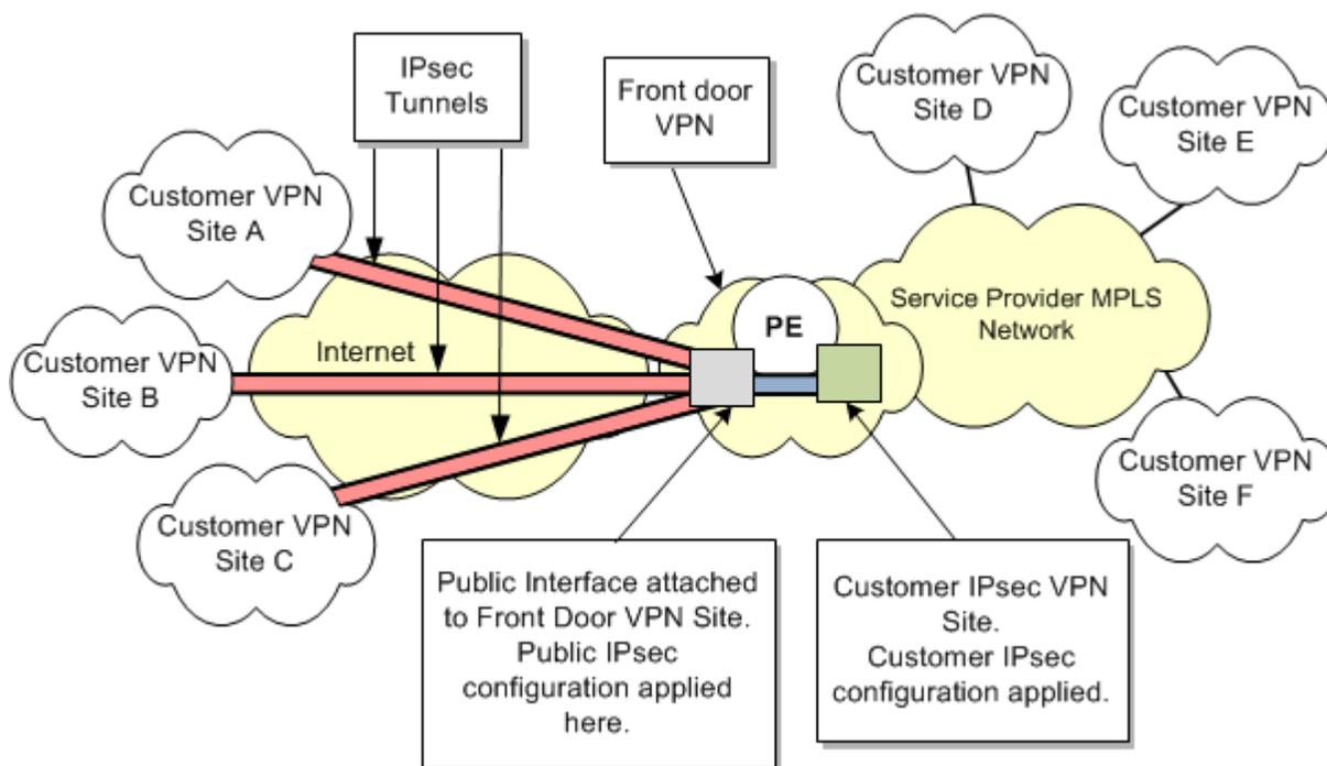
A service provider has an MPLS-enabled core network and provides a customer with VPN access between customer sites D, E, and F.
