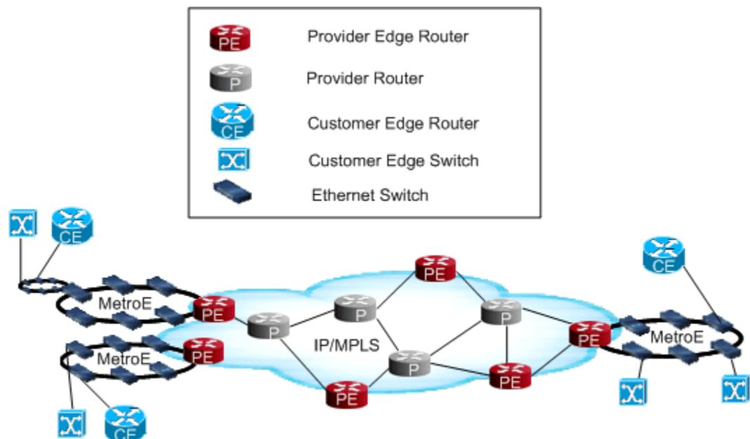
Depending on physical distance, a Metro Ethernet network may be small or large. A small Metro Ethernet network can be a single switch (or two for redundancy if placed in parallel), each connected to their own PE interface on a PE router.
