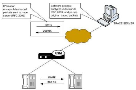
It is possible that—for large frames—when the Oracle® Enterprise Session Border Controller performs the steps to comply with RFC 2003 by adding the requisite header, the resulting packet might exceed Ethernet maximum transmission unit (MTU). This could result in packets being dropped by external network devices, but widespread support for jumbo frames should mitigate this possibility.
