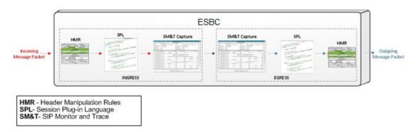
You configure the monitoring process to filter the active session data from original ingress or final egress SIP session messages. The filters are based on the Acme Packet Command Line Interface (ACLI)-configured filters matching criteria or dynamic events that occur, and are used for the purpose of troubleshooting SIP sessions on the network.
