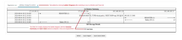
The following screen capture shows an example of an Enterprise SBC ladder diagram with the Session Summary and QoS sections expanded. This screen capture also shows an example of the pop-up that displays detailed SIP Message Details when you hover over a row in the diagram.
