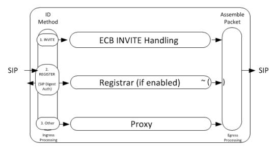
The following diagram displays the key processing elements handling an INVITE, including number normalization, based on context, end station look up, and recursive route set creation.
