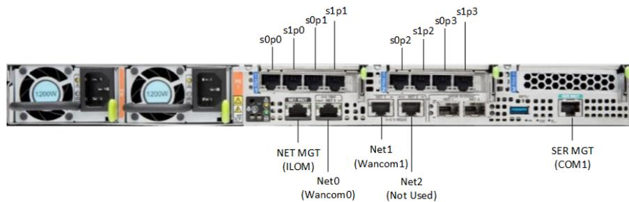
**Figure 1-28 Oracle X7-2 Configuration B (One QSFP and One 4x10 GigE NICs)**
