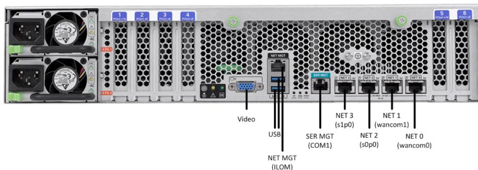
**Figure 1-32 Netra X5-2 for Communications Configuration B (4 Onboard 10 GigE Ports & 1 Quad GigE NIC)**
