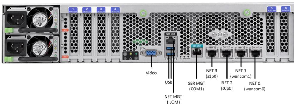
**Figure 1-17 Netra X5-2 for Communications Configuration B (4 Onboard 10 GigE Ports & 1 Quad GigE NIC)**
