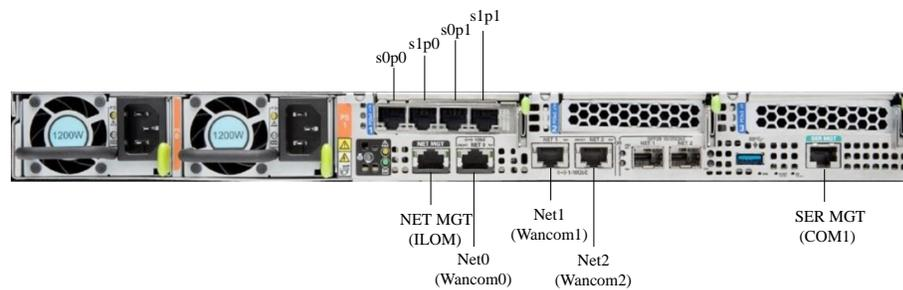
**Figure 1-12 Oracle X7-2 Configuration B (Two 4x10 GigE NICs)**
