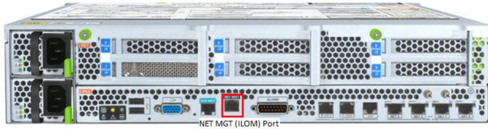
3. Lead the cable away from the rear panel, and connect the other end of the cable to the LAN.
