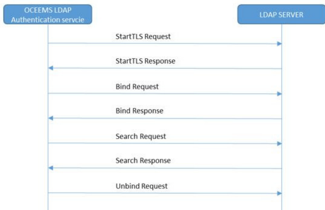
Figure 7-1 Sample Call Flow for LDAP Authentication
