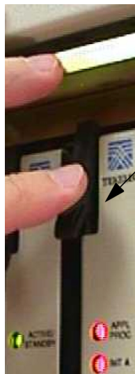
Figure A-12 Push in Inject/Eject Clamps
