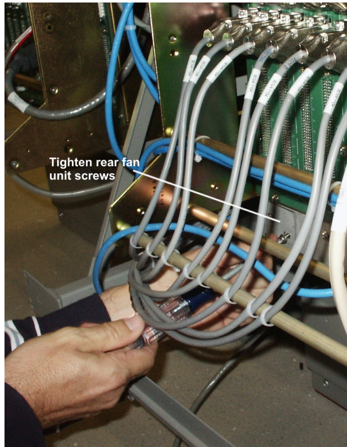
Figure A-23 Tighten rear fan tray screws
