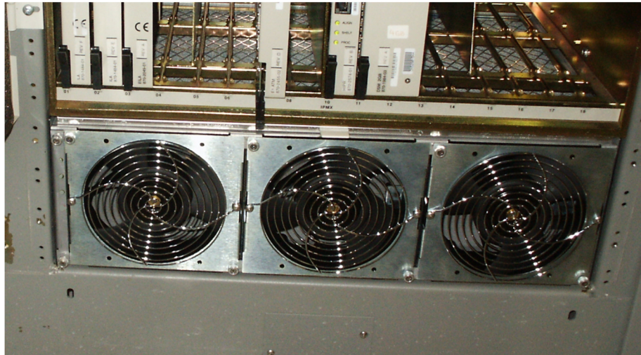
Figure A-22 Fan tray inserted into fan tray bracket in the frame - front view
