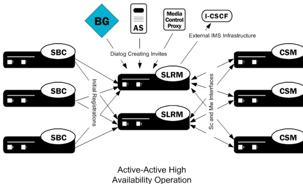
Configuring the devices running SLRM as Session Agents within Session Agent Groups on Oracle SBCs is one method of establishing redundant connectivity. A more generic means of establishing redundant connectivity could be to use DNS techniques, such as dynamic or round-robin DNS, as the means for the P-CSCFs to reach redundant SLRMs.
