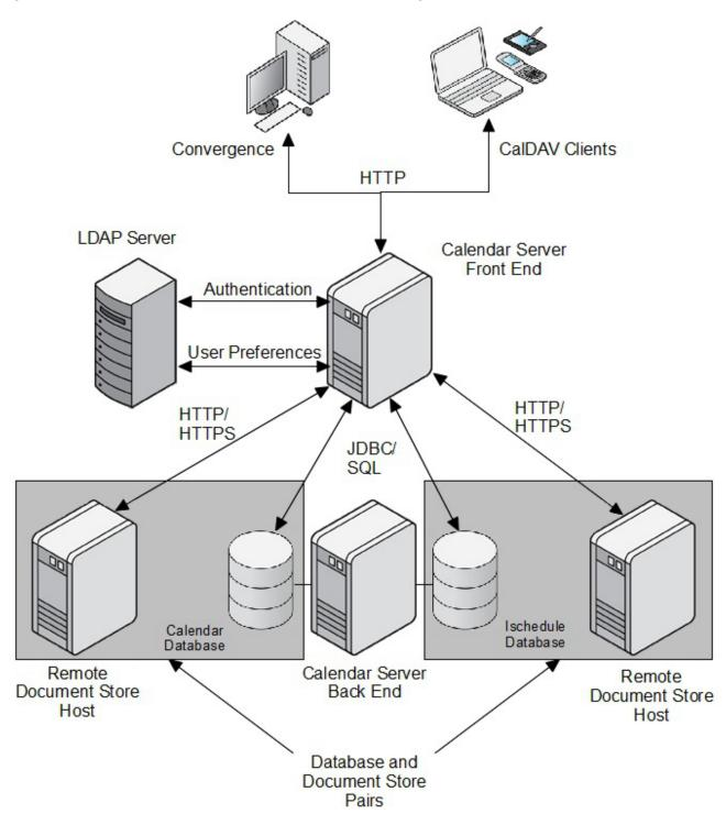
Figure 2-1 Calendar Server Front-End and Back-End Configuration
