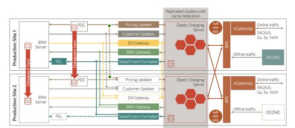
Figure 75-5 Architecture of Active-Active Disaster Recovery System
