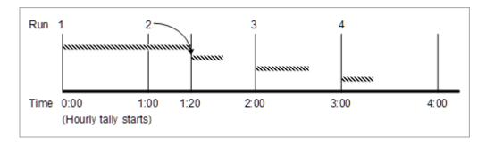
In this example, the first run of **handler4** continues for more than an hour, taking it past the time when the second run is supposed to begin. The second scheduled run cannot start at the one-hour interval, so it starts as soon as possible after that (1:20 a.m.). The third and fourth scheduled executions start at regular multiples of the interval, measured from the first run.
