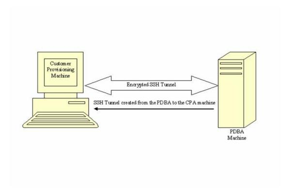
Figure 2-4 SSH Tunnel Between the CPA and PDBA Machines
