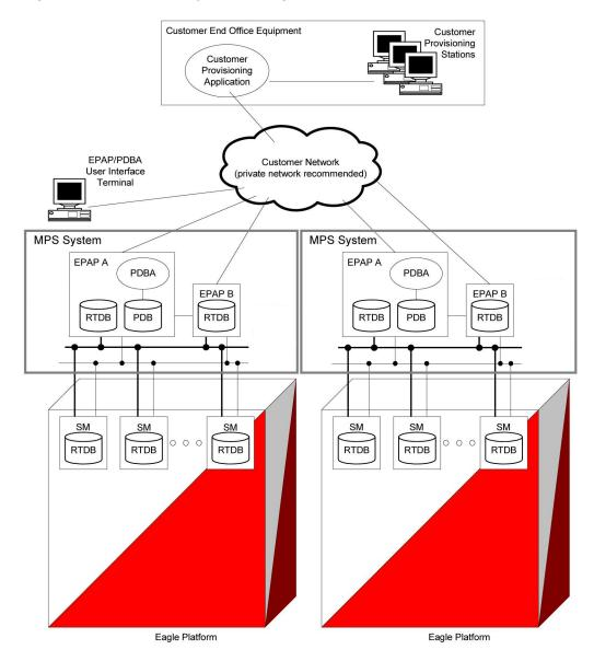
Figure 2-3 MPS/EPAP System Configuration
