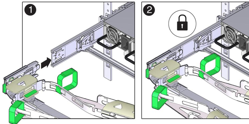
8. Gently tug on the four CMA connection points to ensure that the CMA connectors are fully seated before you allow the CMA to hang by its own weight.
