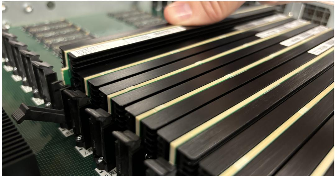
4. Press on the latches on both sides to secure the TM to the mainboard.
