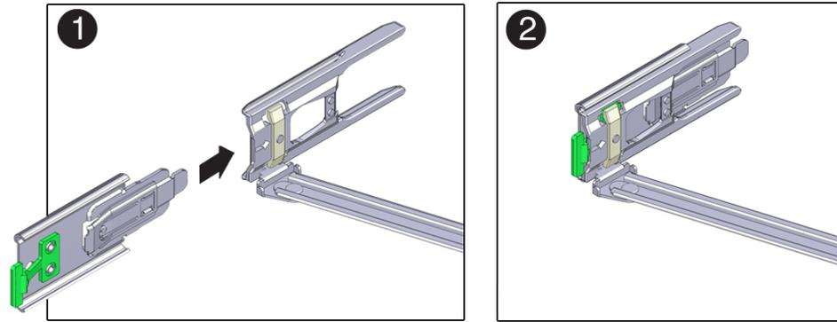
7. To install CMA connector D into the left slide-rail:
