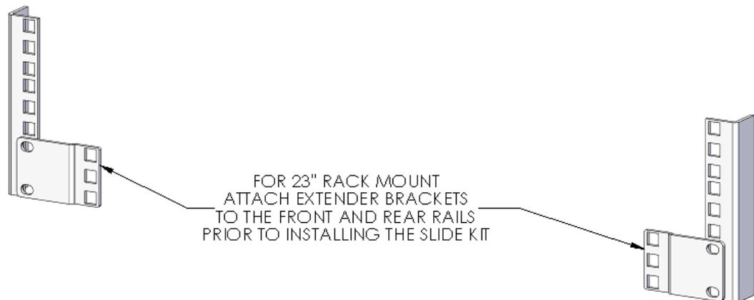
2. Attach the 23" Center Mount Brackets to the Acme Packet 6400.
