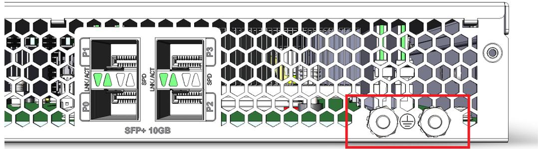
2. Place the lug on the end of the grounding cable onto the grounding posts.
