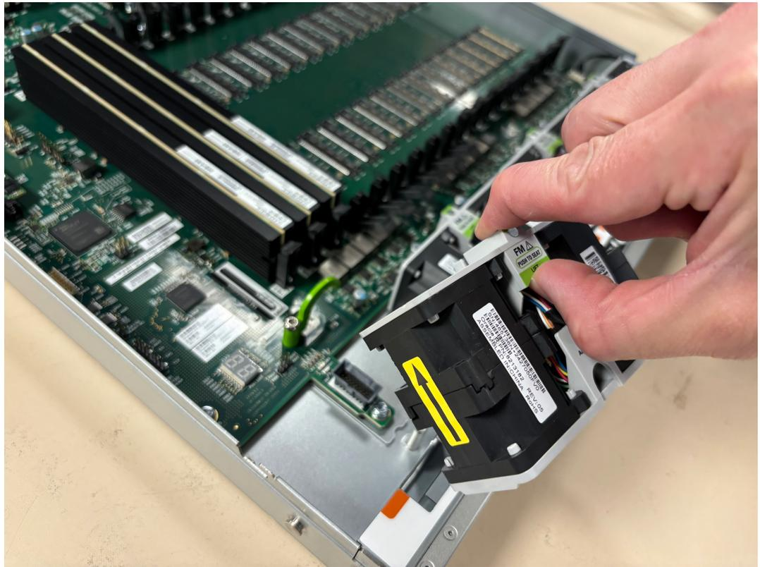
2. Press down to secure and attach the fan module.
