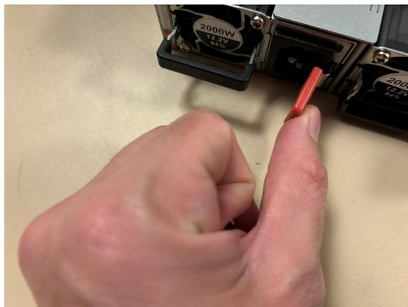
3. Holding the handle, pull the power supply towards you. This will disengage the power supply from the chassis.
