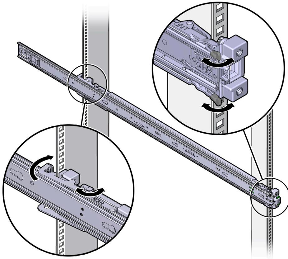
3. Align the front of the slide-rail assembly against the outside of the front rack rail, and push until the assembly locks into place with an audible click.
