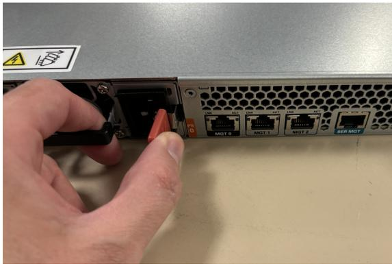
4. Continue pulling the power supply towards you until it is completely removed from the chassis.
