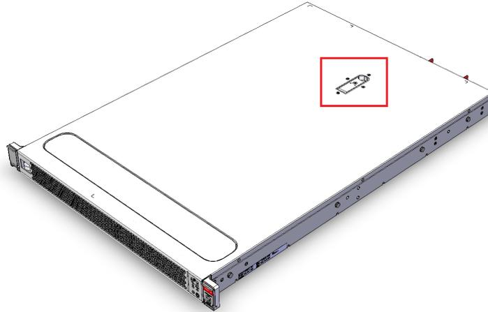
2. Use a T15 Torx tip screwdriver to unlock the latch.
