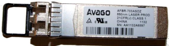
The following image shows the single mode 10 gigabit SFP+ transceiver used in the Acme Packet 6400.
