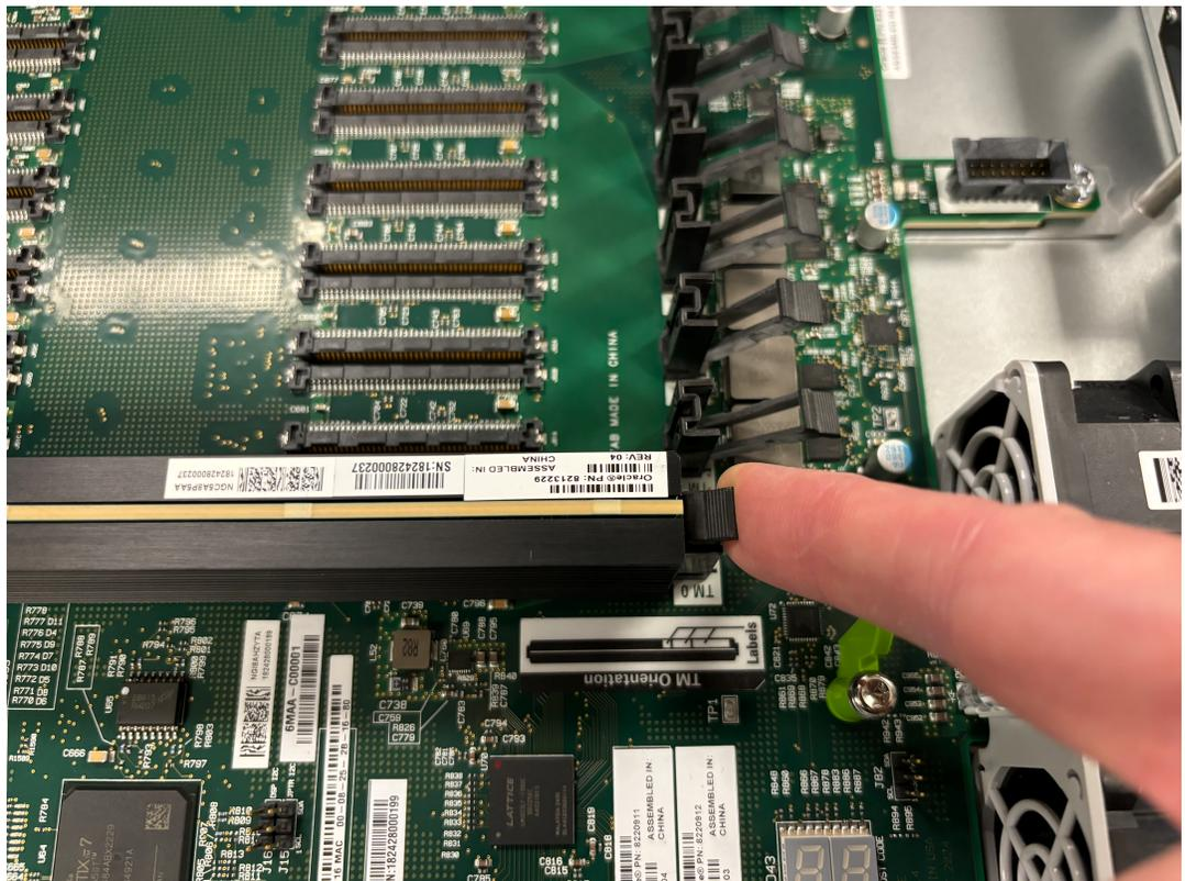
5. As necessary, repeat for slots TM1, TM2, and others, making sure to install the TMs sequentially.
