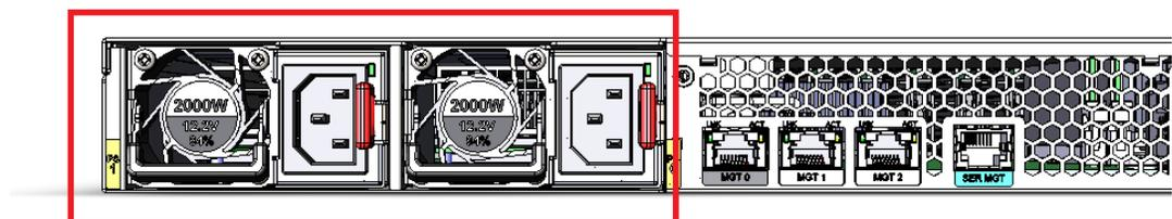
3. Connect the other power cord to the AC power supply by inserting the 3-lead IEC-320 plug into the IEC connector located on the power supply.
