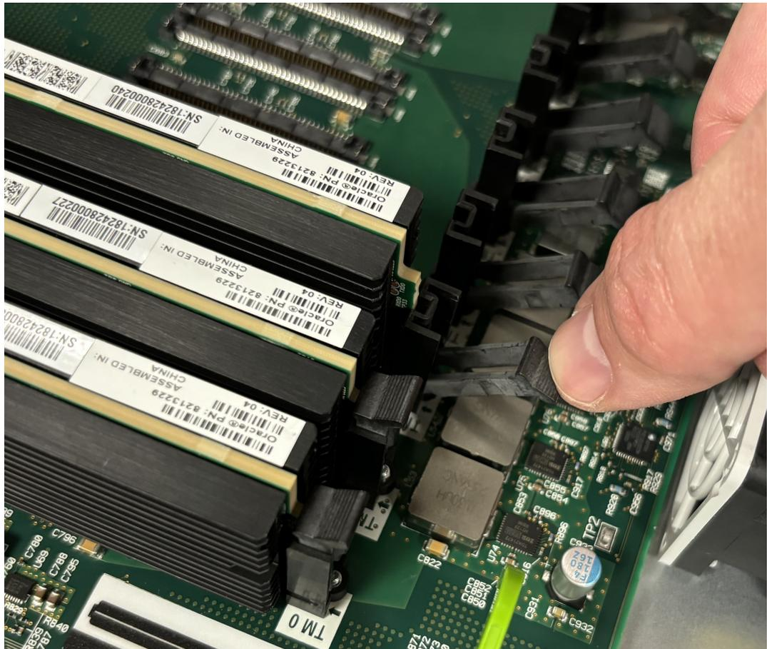
4. When both sides are free of the latch, hold the center of the module between your finger and thumb and slowly remove the module. Be careful to keep the module level while removing it and guide it smoothly through the guide slots on either side.
