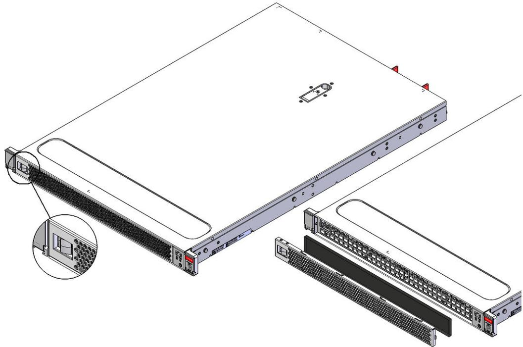
2. Gently wipe the front fan bezel that contains the perforated air inlets with a clean, dry cloth. Alternatively, use compressed air to clean out the perforated air inlets.
