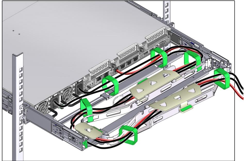
13. Ensure that the secured cables do not extend above the top or below the bottom of the Acme Packet 6400 to which they are attached.
