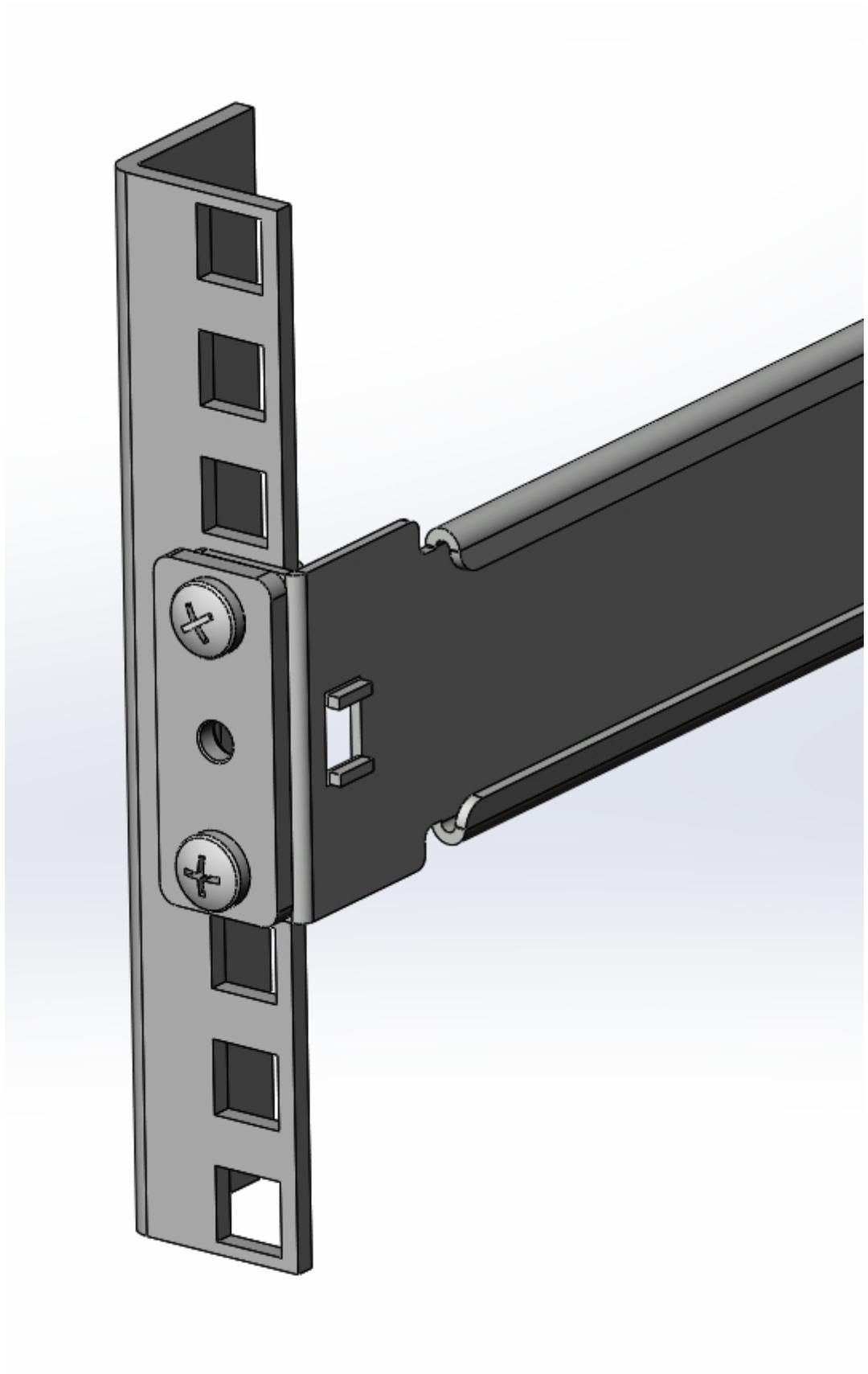
Stationary Slide Rail Secured to Front Mount Point
