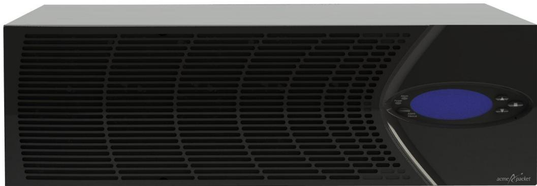
Dark Graphic Display When Acme Packet 6300/6350 is Shut Down
