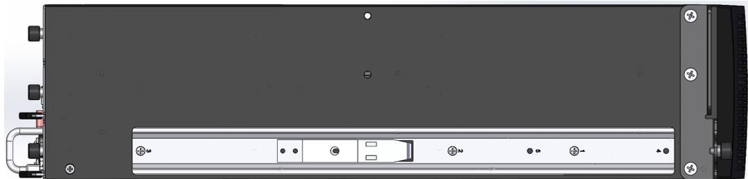
Chassis Slide Rail Installed
