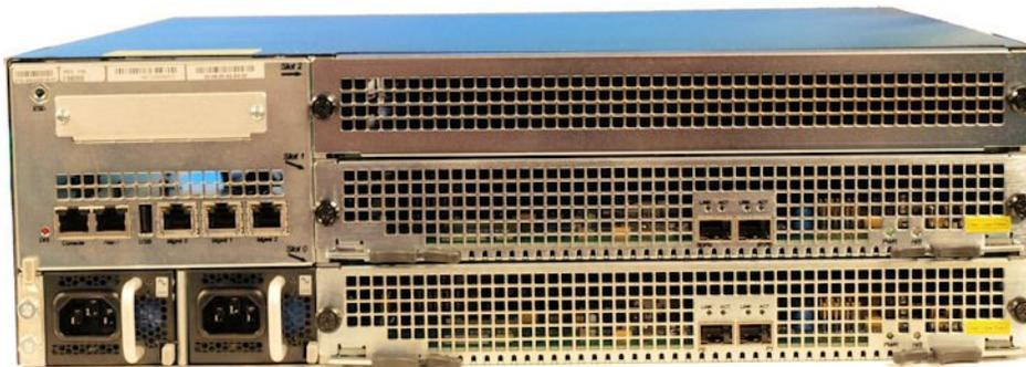
Figure 2-3 Typical Option Card - Two Port NIU
