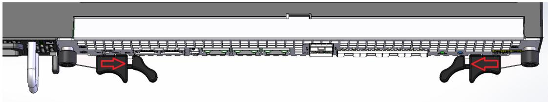
5. Slide the lever catch and pivot the two ejector levers outward at the same time, pulling the card out of its connection to the motherboard and away from the system chassis. This action disengages the NIU/TCU from the system, severing all electrical contact to the processing unit.
