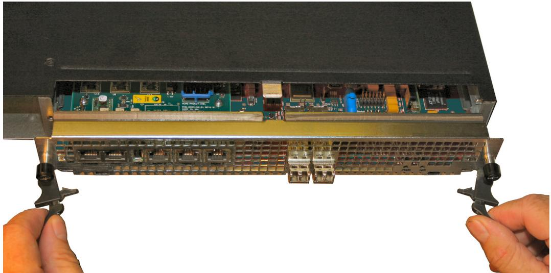
Installing the NIU/TCU (NIU Shown)
