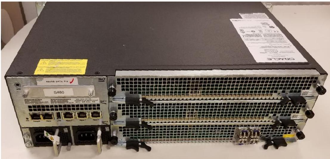
**Figure 2-5 Alternate Option Card - Four Port NIU**
