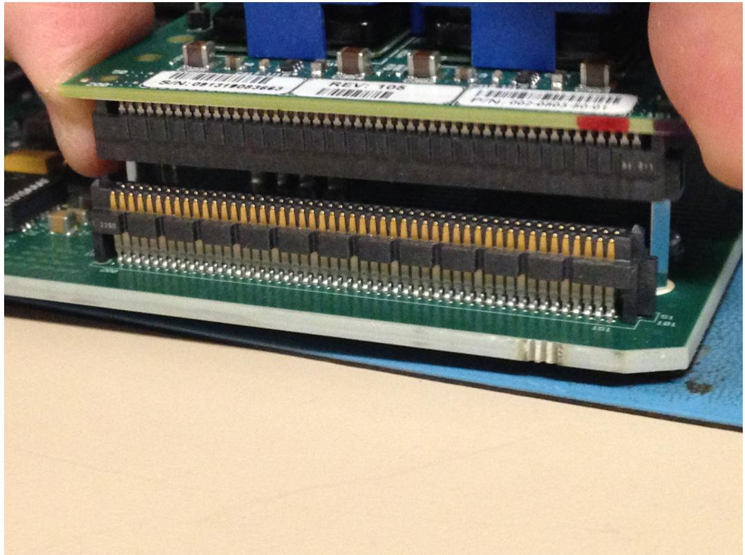
Installing the SSM3 Module
