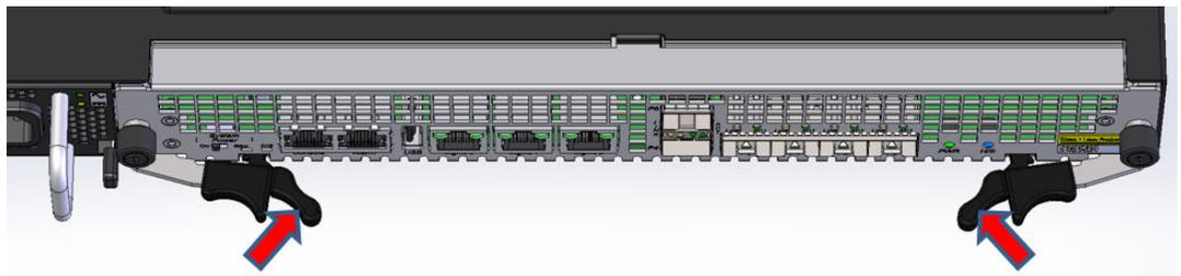
Ensure pressure is applied to the ends of the ejector (not the sliding section) when seating the NIU/TCU
