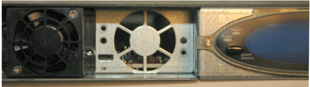
**Figure 6-5 Inserting the Fan into the Chassis Slot**
