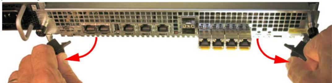
6. Remove the loosened NIU/TCU out of the Acme Packet 6300/6350 by holding and pulling on each side of the NIU's front panel.
