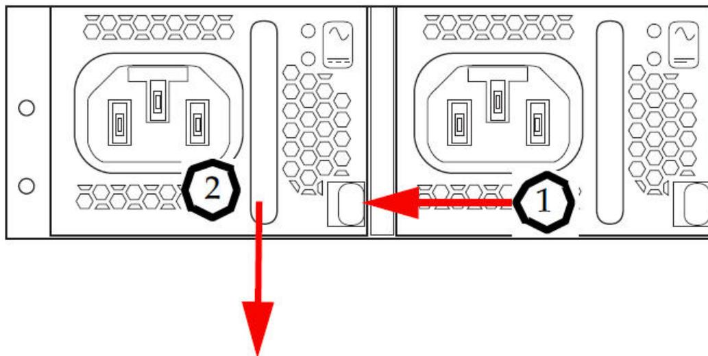
3. Holding the handle (2), pull the power supply towards you. This will disengage the power supply from the chassis.
