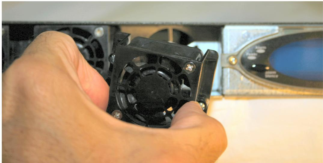
2. Using a small bladed screwdriver, tighten the two captive screws to hold the fan into place.
