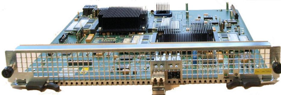
Installed SFP+ Transceiver
