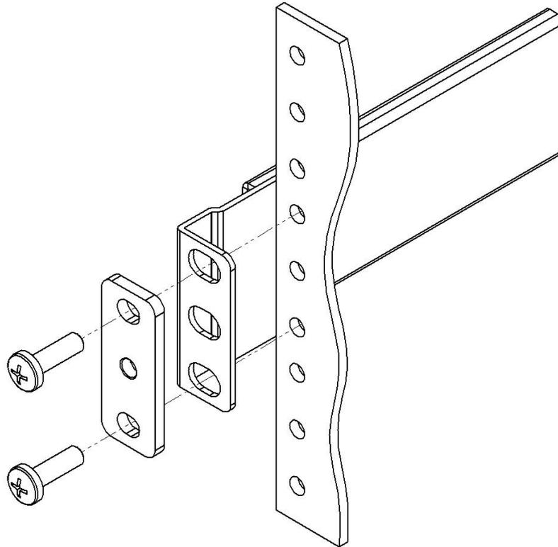
Screwing In and Securing the Stationary Slide Rail
