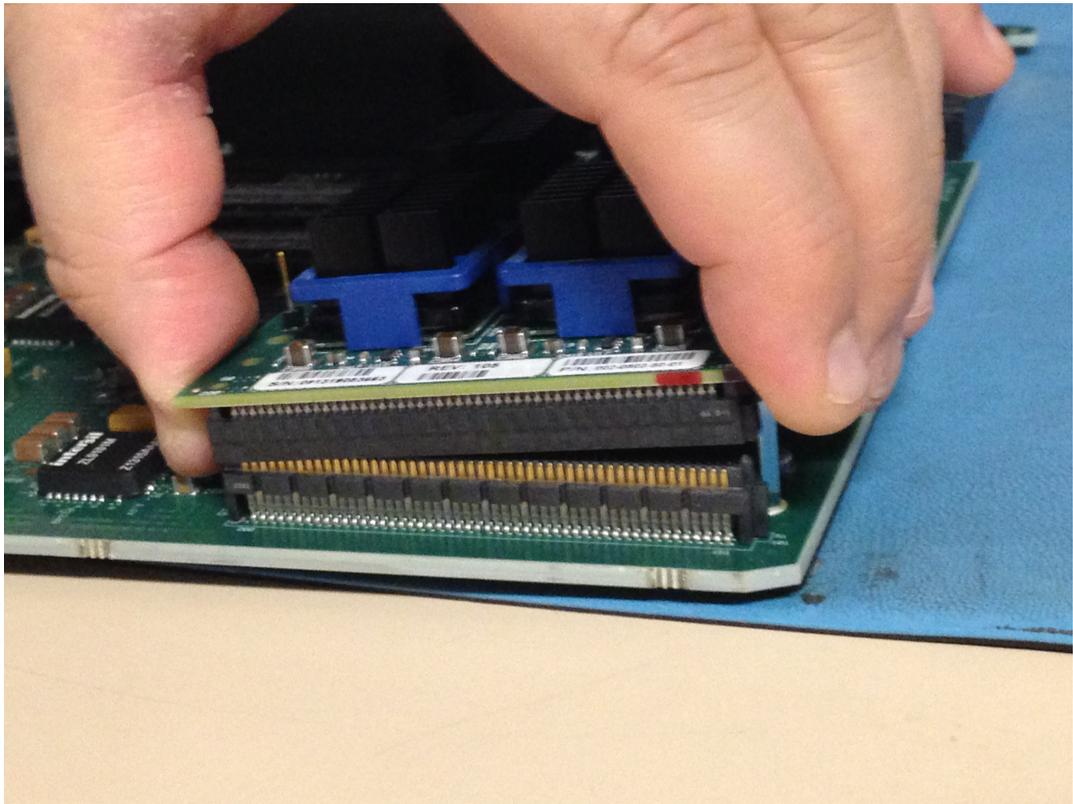
Removing the SSM3 Module
