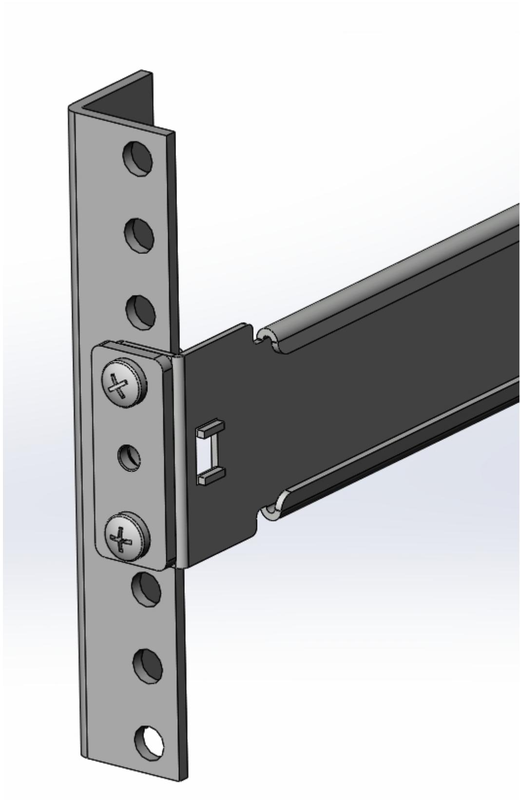
Installed Stationary Slide Rail
