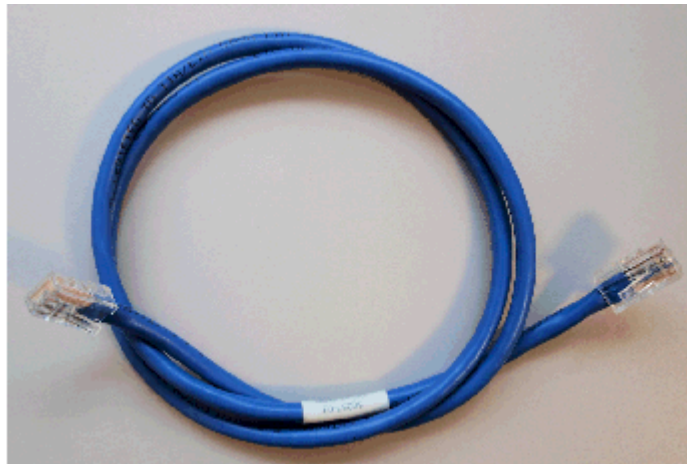
A copper transceiver uses Category 5 or 6 Ethernet cable.
