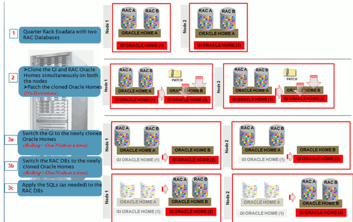
Figure 14-8 Out Of Place Patching Of Clusters
