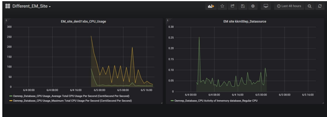
Dashboard with a single panel pulling data from a different Enterprise Manager sites (Data from multiple Enterprise Manager sites , single panel):
