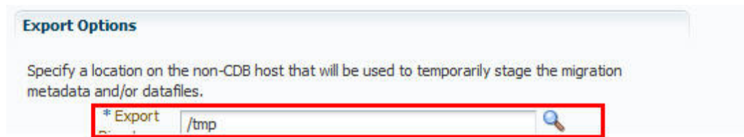
Figure 13-32 Migrating a Non-CDB: Specifying Stage Location
