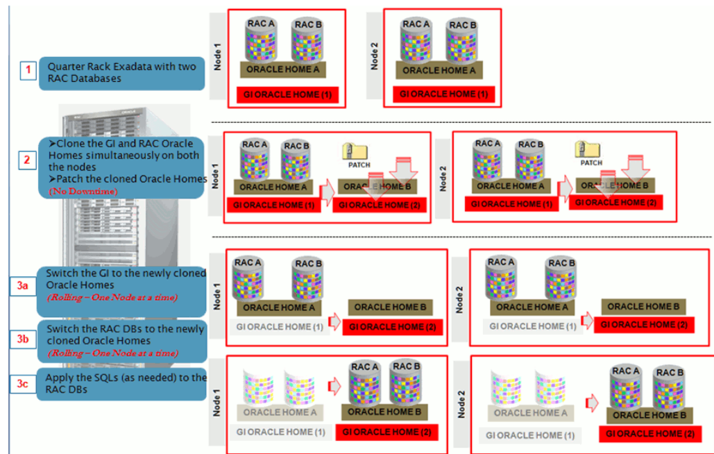
Figure 21-10 Out Of Place Patching Of Clusters
