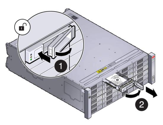
3. Install the replacement drive by opening the drive lever on the replacement drive. Slide the new drive into the drive slot [1] until it engages with the backplane connector and then close the lever to fully seat the drive and lock it into place [2] as shown in the following figure.
