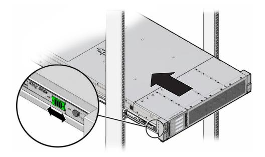
**c.** Continue pushing the server into the rack until the slide-rail locks (on the front of the server) engage the slide-rail assemblies.
