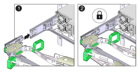
8. Gently tug on the four CMA connection points to ensure that the CMA connectors are fully seated before you allow the CMA to hang by its own weight.
