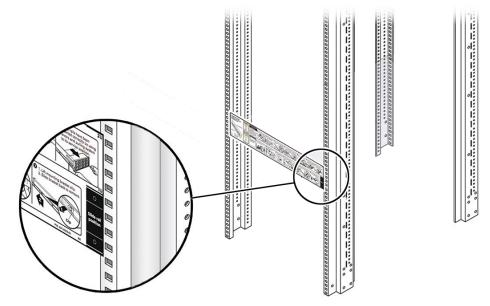
3. Mark the mounting holes for the front slide-rails.
