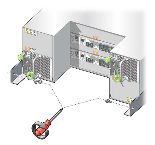
**10.** Attach AC power cords to the storage shelf power supplies and to the rack PDUs (Power Distribution Units).
