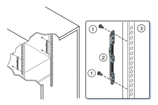
The following figure shows the rear adapter brackets being attached to a square-hole rack:
