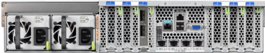
Figure 3-34 Rear View of Extreme Flash Exadata Storage Server X5-2 Servers
