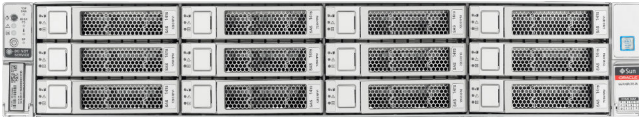
Figure 3-19 Front View of Oracle Exadata Storage Server X8M-2 and X8-2 High Capacity and XT servers
