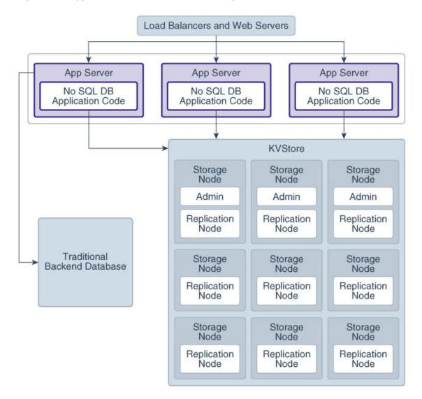
Figure 1-1 Typical Architecture for Oracle NoSQL Database Store
