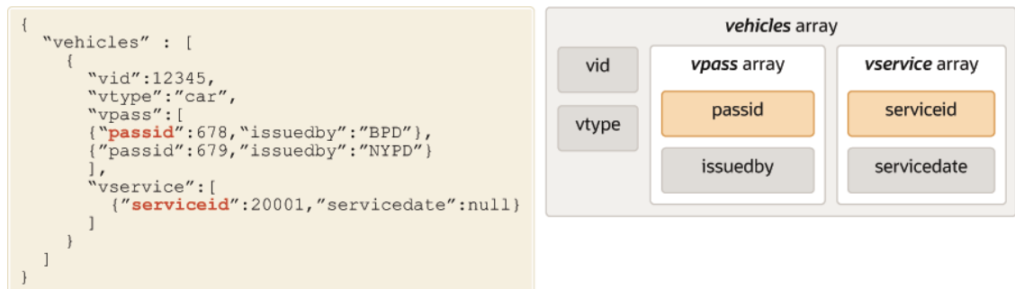
Figure 8-4 Composite Multikey Index (invalid)
