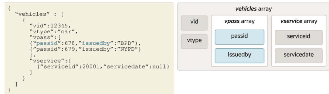
Figure 8-2 Composite Multikey Index
