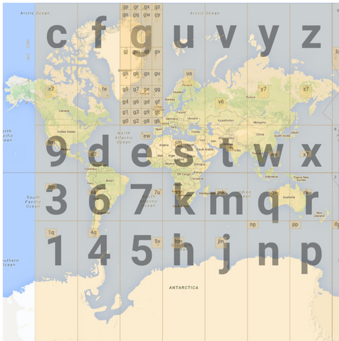
Figure 11-5 Level-1 and Level-2 Geohash Cells
