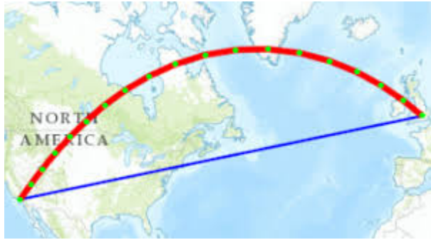
Figure 11-1 Geodetic vs Straight Line
