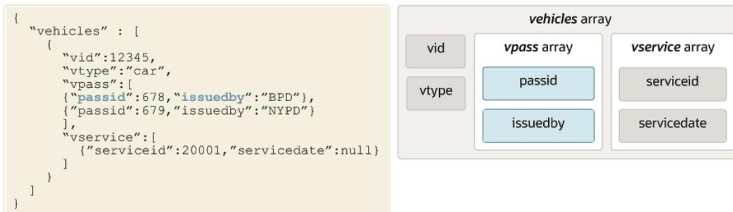
3. You can use fields of an array/record/maps-viewed-as-records, as well as the fields present inside the inner arrays of those array/record/maps-viewed-as-records together. However, the restriction here is that the immediate parent array of all such fields should be the same.
