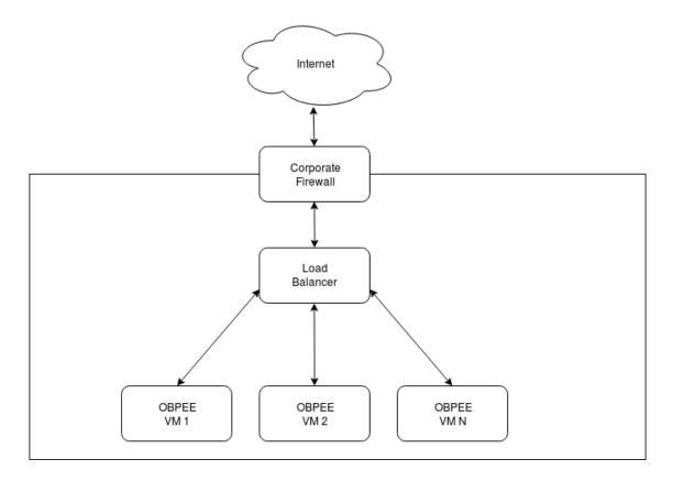
Figure 1-2 Firewall, load balancer, and instance relationship
