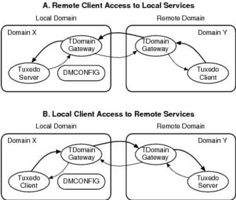
In the example, you must also create a `DMCONFIG` file for Domain Y that complements the `DMCONFIG` file created for Domain X. That is, a local domain access point in the Domain X `DMCONFIG` file would be a remote domain access point in the Domain Y `DMCONFIG` file, and a remote domain access point in the Domain X `DMCONFIG` file would be a local domain access point in the Domain Y `DMCONFIG` file. The example demonstrates the use of the TDomain gateway server.
