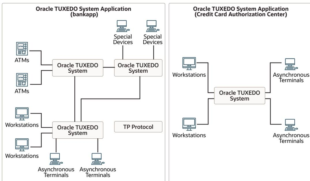
To create the Domains configuration for the `bankapp` and credit card authorization applications, you need to create two `UBBCONFIG` files, one for each of the Oracle Tuxedo applications, and two `DMCONFIG` files, one for each of the Oracle Tuxedo applications.
