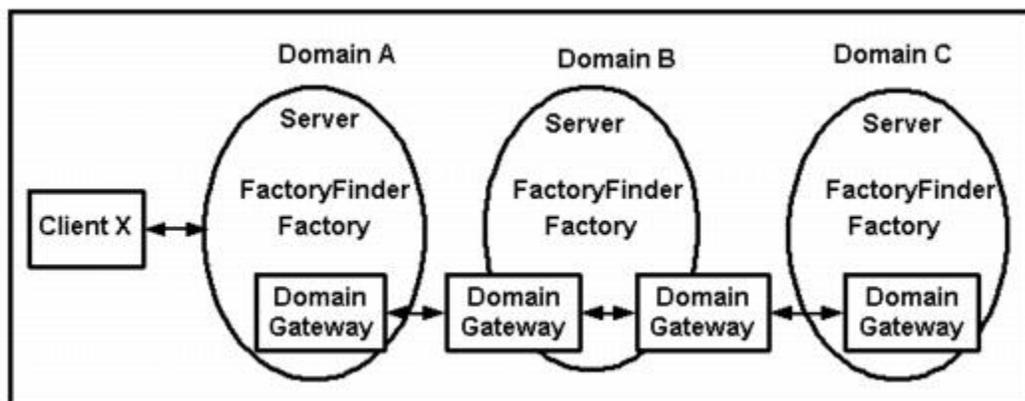
Domains A and B are directly connected, and Domains B and C are directly connected, but A and C are not directly connected. For Domains A and C to communicate, they must use Domain B as the intermediary. Therefore, the `DMCONFIG`
