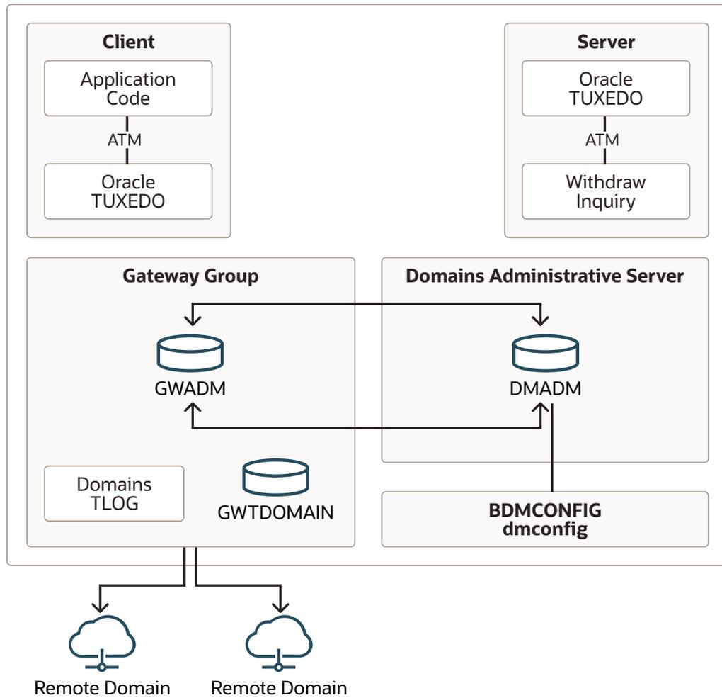
A domain *gateway group*, as shown in the previous figure, consists of a *gateway administrative server* (GWADM), a domain gateway server (for example, GWTDOMAIN), and (optional) a Domains transaction log (TLOG). The GWADM server enables run-time administration of the domain gateway. An Oracle Tuxedo domain can communicate with one or more remote domains through a domain gateway group.
