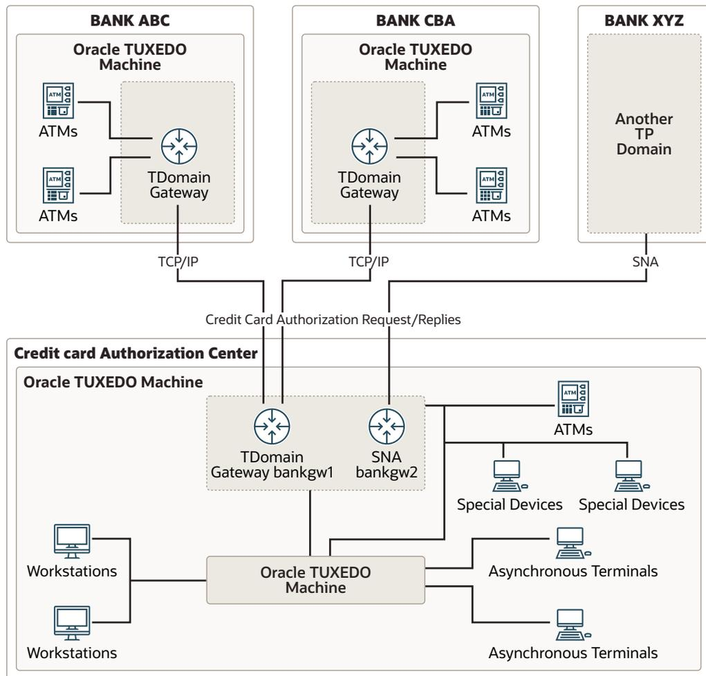
The Oracle Tuxedo credit card authorization center at the bottom of the figure has two gateway groups: a TDomain gateway group named `bankgw1` and a SNA gateway group named `bankgw2`. `bankgw1` provides access to two remote Oracle Tuxedo domains, Bank ABC and Bank CBA, using network protocol TCP/IP. `bankgw2` provides access to one remote domain, Bank XYZ, using network protocol SNA.
