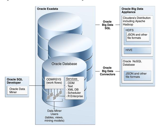
Figure 1-1 Oracle Data Miner Architecture for Big Data
