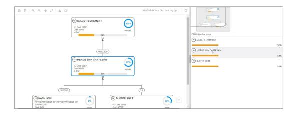
The diagram navigator shows a list with steps having more than 1% CPU cost in descending order. Click a step in the list to navigate to the same step in the diagram, enabling you to see it in the context of the other steps.
