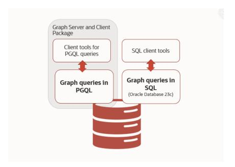
Figure 1-2 Property Graph Architecture for Running Graph Queries
