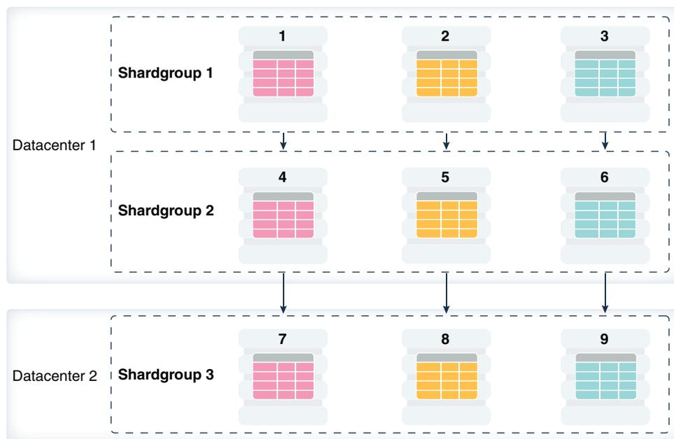
Shardgroup 1 consists of Oracle Data Guard primary databases (shards 1, 2, 3). Shardgroup 2 consists of local standby databases (shards 4, 5, 6) which are located in the same datacenter and configured for synchronous replication. And Shardgroup 3 consists of remote standbys (shards 7, 8, 9) located in a different datacenter and configured for asynchronous replication. The default replication topology is Oracle Data Guard. To open each standby in
