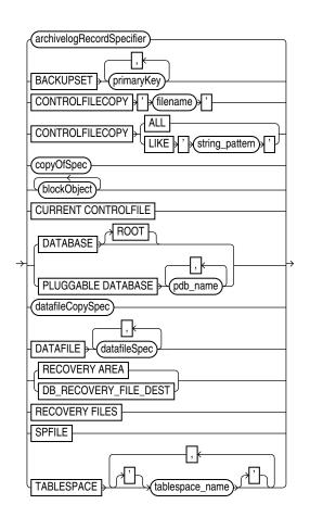
(archivelogRecordSpecifier::=, copyOfSpec::=, blockObject::=, datafileCopySpec::=, datafileSpec::=)
