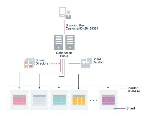
Figure 1-5 Oracle Globally Distributed Database Architecture
