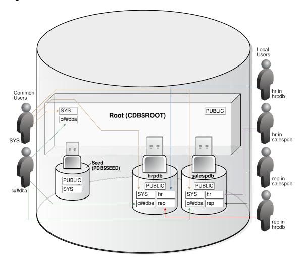
Figure 4-3 Users and Schemas in a CDB
