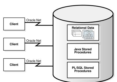
Figure 11-4 Two-Tier Client/Server Configuration
