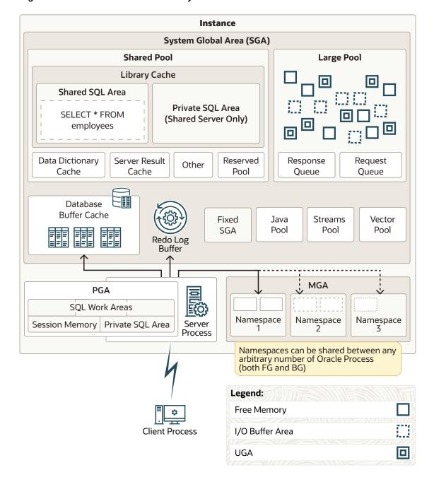
Figure 17-1 Oracle Database Memory Structures
