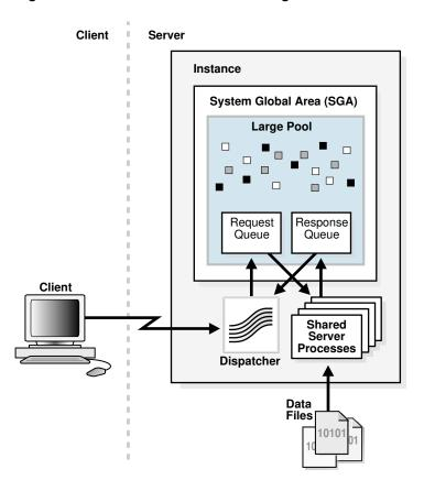
Figure 19-9 The Shared Server Configuration and Processes
