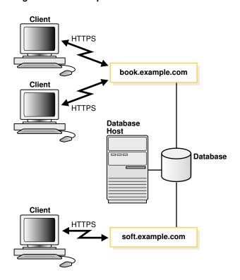
Figure 19-6 Multiple Services Associated with One Database
