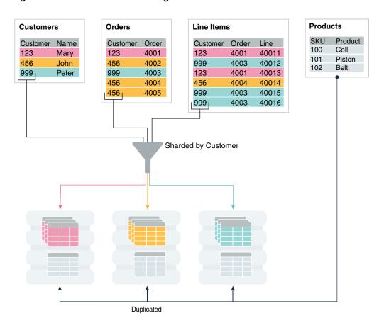
Figure 6-7 Horizontal Partitioning of a Table Across Shards
