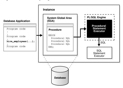
Figure 11-3 The PL/SQL Engine and Oracle Database
