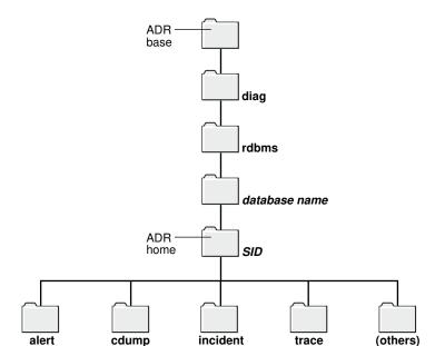
Figure 16-8 ADR Directory Structure for an Oracle Database Instance
