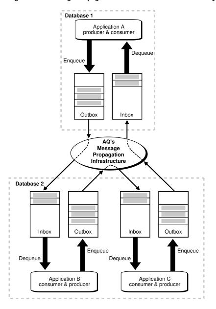
Figure 1-9 Message Propagation in Oracle Database Advanced Queuing
