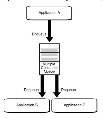
Figure 1-3 Communication Using a Multiconsumer Queue
