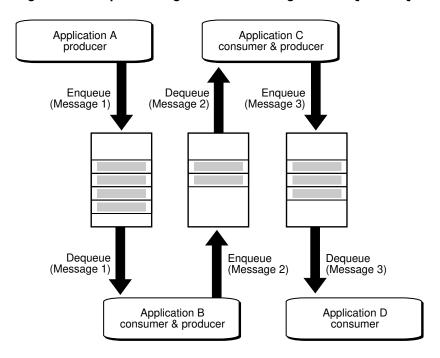
Figure 1-5 Implementing a Workflow using TxEventQ and AQ
