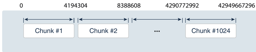
Figure 2-6 Ranges of Hash Values Assigned to Chunks
