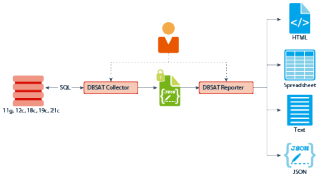
Figure Collector and Reporter Components and Architecture
