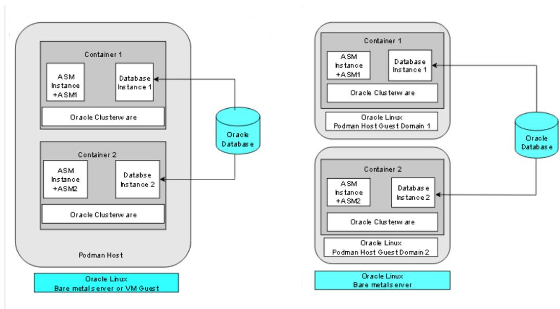
For virtual test and development clusters, you can use two or more Podman containers as nodes of the same cluster, running on only one Oracle Linux Podman host, because high availability is not required for testing.
