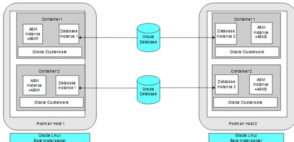
The following figure shows another production deployment, in which containers are located in different Podman hosts on separate hardware servers, with a high availability storage and network configuration:
