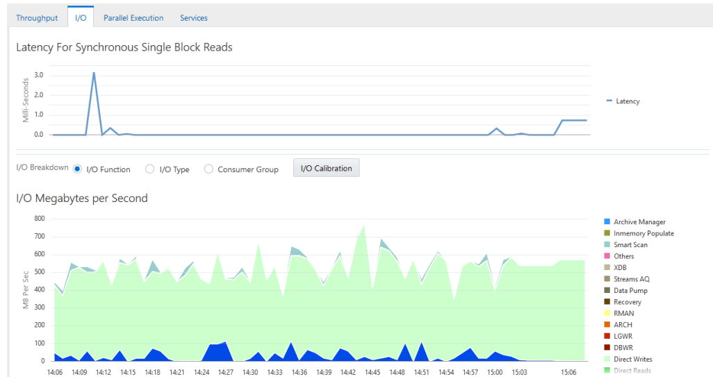
Figure 4-5 Performance Monitoring I/O by Type
