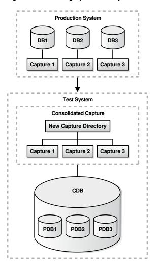
Figure 15-1 Setting Up the Test System for Consolidated Database Replay
